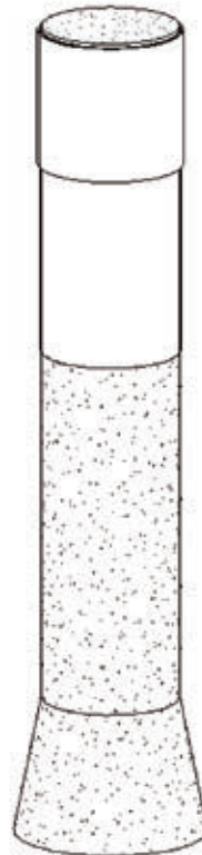
Fig 4.2.1 – 3D View of Bored Pile
