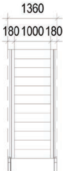
Figure 16.4.2 – Plan View of Metal Stair
