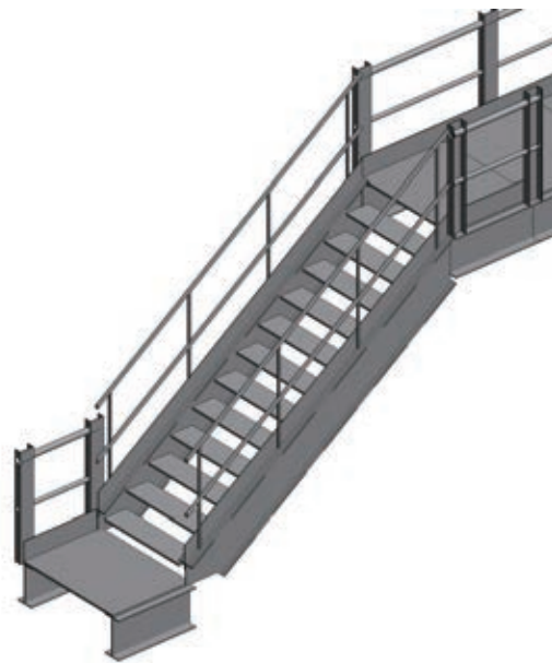
Figure 16.4.1 – 3D View of Metal Stair
