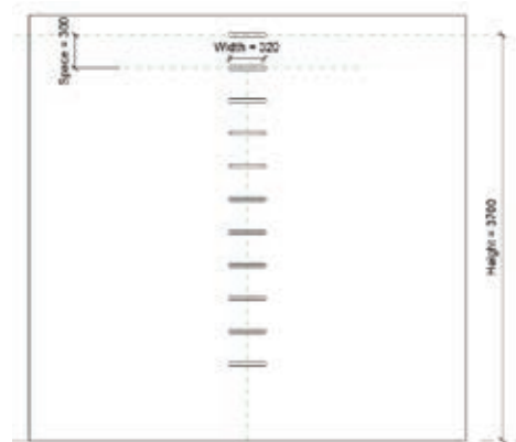
Figure 17.3.3 – Front Elevation of Step Irons
