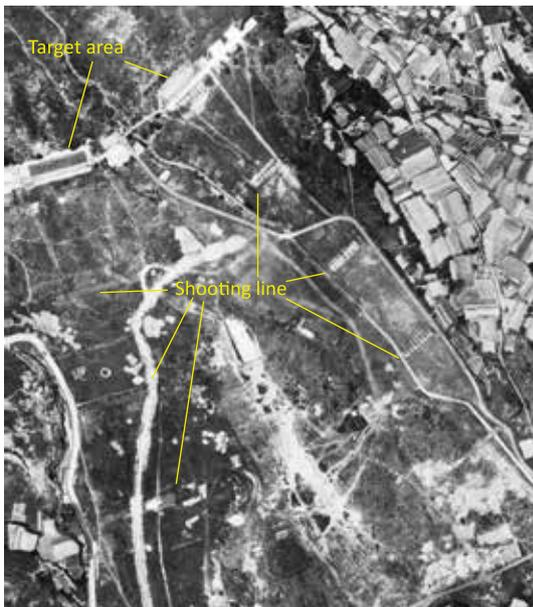
**Figure 15:** Kowloon City Rifle Range in 1949. The stop butts and galleries are at the top left. The built up firing points are at 100 or 200 yard intervals extending back to the maximum range limits (Portion enlargement of R.A.F. aerial photo No. 6056 81A 130).
