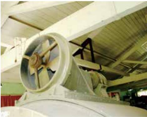
**Figure 7:** Ventilation fan on top of the searchlight helped dissipate heat and smoke generated by the electric arc (Photo by author in 2010).
