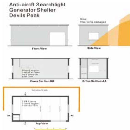
**Figure 108:** Different aspect views of the AASL generator shelter.
