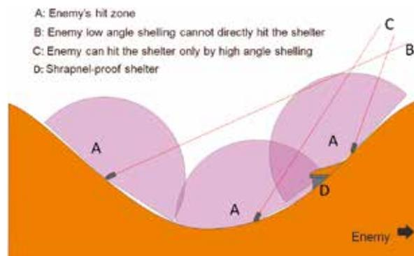
**Figure 6:** HQ shelter protected by hiding it in a valley.
