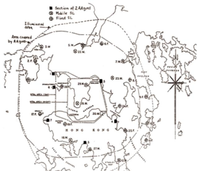
Figure 1: The Anti-Aircraft Gun and Searchlight layout as planned in 1937.
