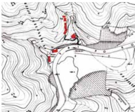
**Figure 38:** HQ buildings highlighted on a 1963 survey map. Note that the map shows the original Tai Po Road curved around the hill, which has since been straightened. The dotted line shows part of the old Tai Po Road after straightening (1963 1:1200 C-145-SW-D).
