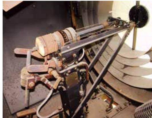
**Figure 6:** The carbon rods inside the searchlight generated highly luminous electric arcs when the power was on. The rack of horizontal carbon rods can adjust the position between two carbon rods to generate electric arcs, the arc strikes between the tips of the two rods and the 'rack' is the mechanism for moving the movable rod to the fixed rod as its carbon is consumed during operation. (Photo by author in 2010).
