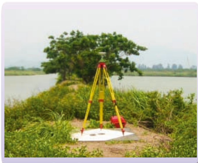
▲ Figure 3 : GPS receiver set-up at Control Point 6 (Picket Box)
