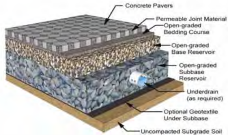
Figure 8.9 Typical Details of Permeable Paving Systems 46
