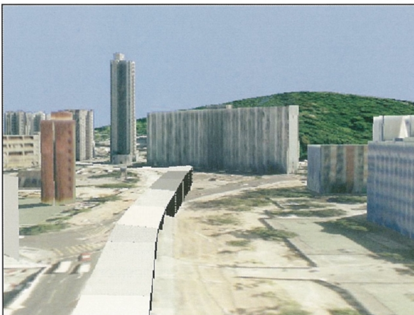
Figure 2 : 3-D Visualization of City Model Produced by Digital Photogrammetry (Courtesy : SMO, HKSAR Government)
