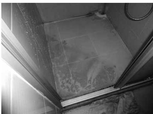
Photo 2 – Fluorescent dye test
