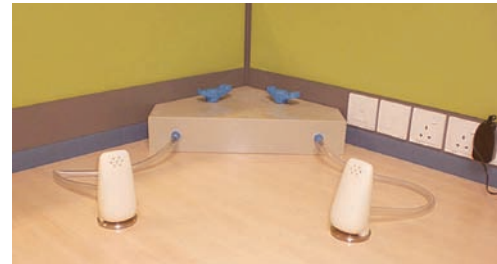
Figure 15: Personalized Ventilation System
